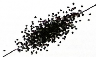
Fig. 1. Principal Component Analysis of a bidimensional data cloud. The line shows the direction of the first principal component.
